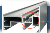
Azo-Brader™ Technology: Abrasion "hooks" displace metal along the lugs to improve adhesion in the thermal barrier pocket.
